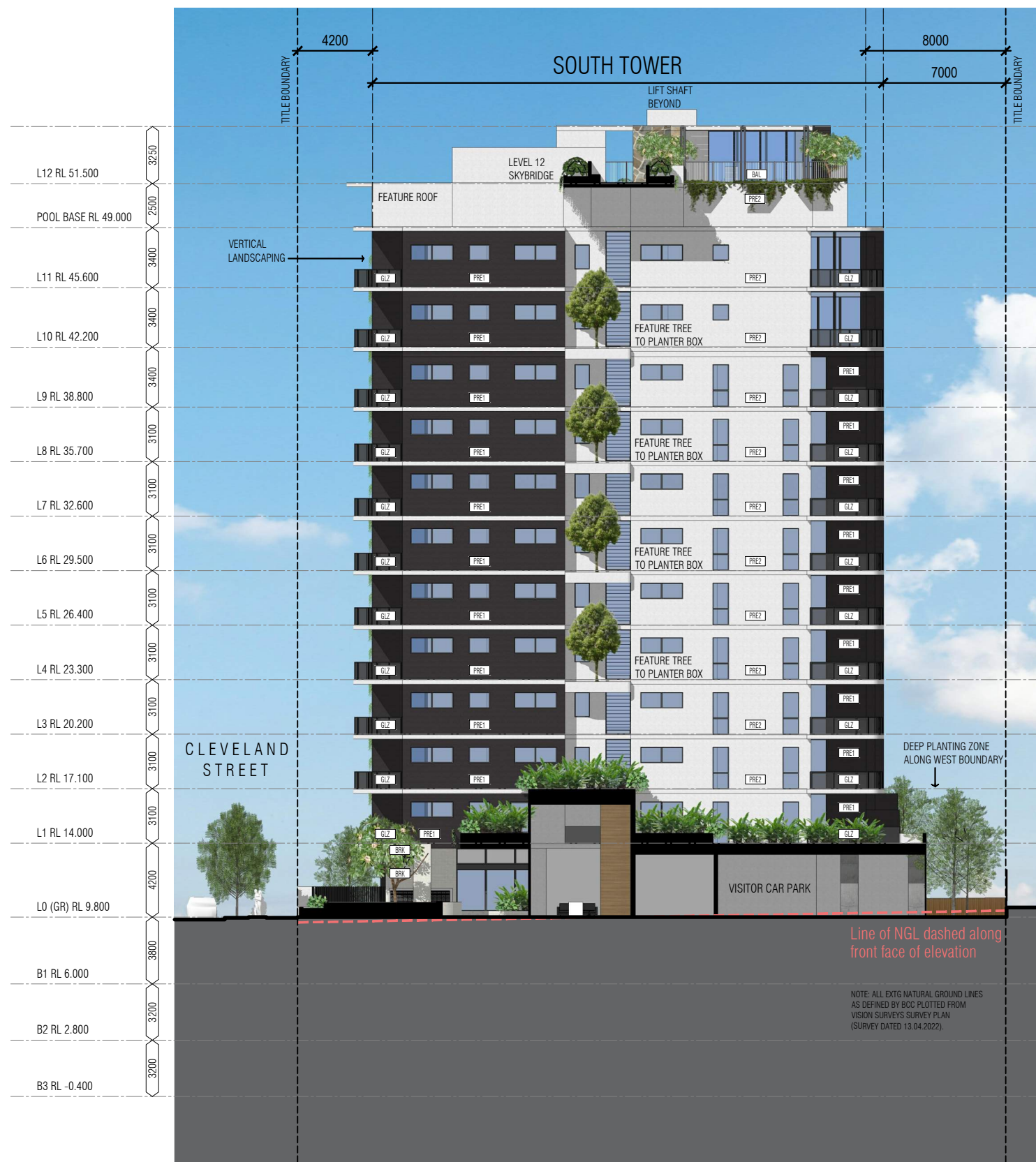
5 INTERNAL ELEVATION (NORTH) 200 1:300@A3
